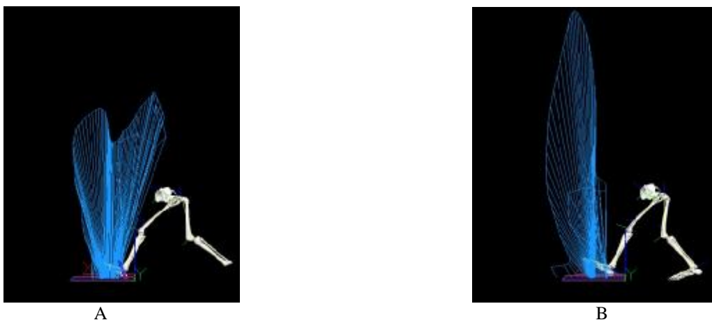
Fig. 3. Vector plot of resultant support reaction when walking by the method of repulsion (A) and attraction/repulsion (B) [3]
